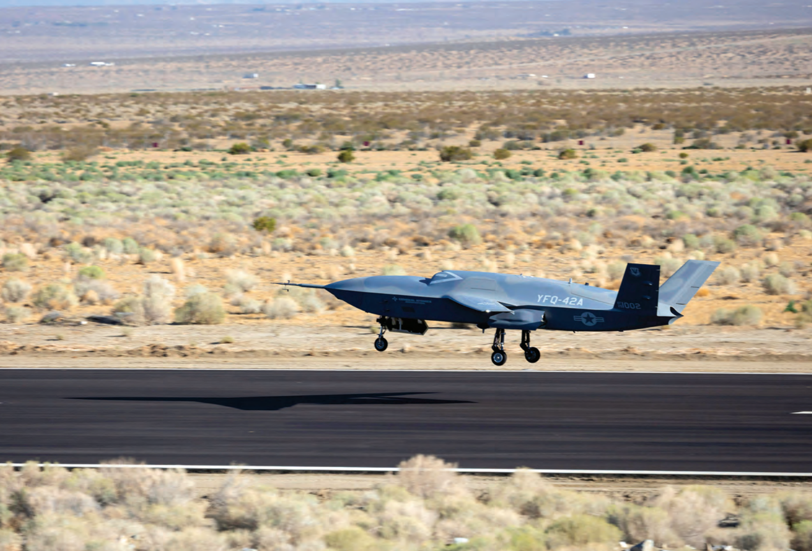
Unmanned combat aerial vehicle YFQ-42A Collaborative Combat Aircraft, developed in partnership with General Atomics, conducts flight testing in California, August 27, 2025 (Courtesy General Atomics)
